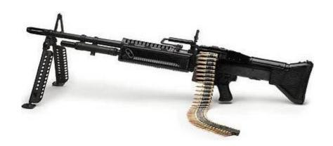
The M-60 machine gun was a belt fed, gas operated, full automatic, gun which fired a .308 caliber or 7.62 mm cartridge.
